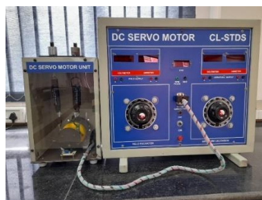
Fig. 3: DC Servo Motor Trainer kit: Control unit and Motor unit.
