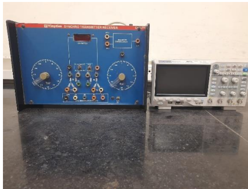
Fig.5 : Synchro Transmitter &amp; Receiver kit and DSO.
