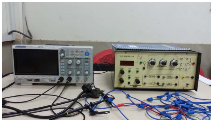
Fig. 1: PID control kit with DSO.
